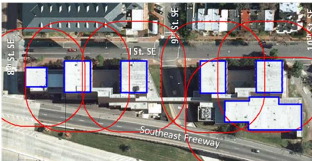
Building 20, aerial view with required standoff distances shown in red
